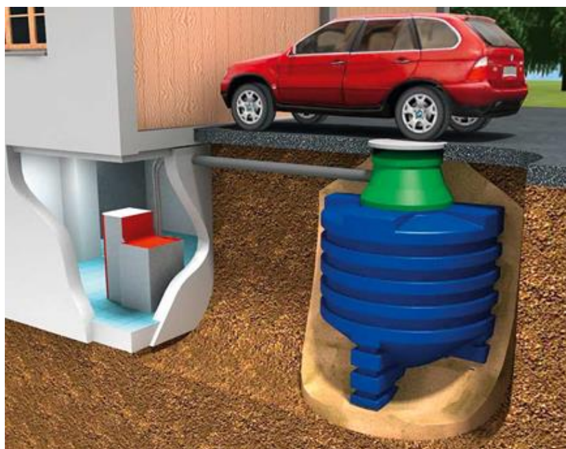
Sl. 5-31 Ukopani spremnik peleta [Froling]
